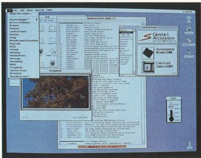
Photo 1: The Macintosh interface contains all the elements of a typical GUI. The pointer (upper left) lets you make selections and position the cursor. Menus supply you with choices among a range of actions. Windows display the output of programs.
